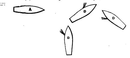
If A sees a White masthead Light above the Red Light, A knows that the vessel is a steam-vessel, and is either approaching her in the same direction, as B, or is crossing to port in some direction, as D D D.
