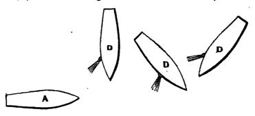
If A secs a White masthead Light above the Green Light, A knows that the vessel is a steam-vessel, and is either approaching her in the same direction as B, or is crossing to starboard in some direction, as D D D.
