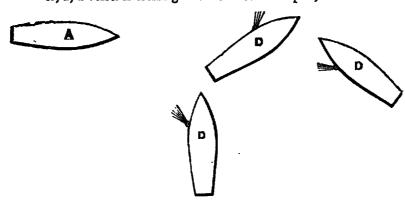
If A sees a White masthead Light above the Red Light, A knows that the vessel is a steam-vessel, and is either approaching her in the same direction, as B, or is crossing to port in some direction, as D D D.
