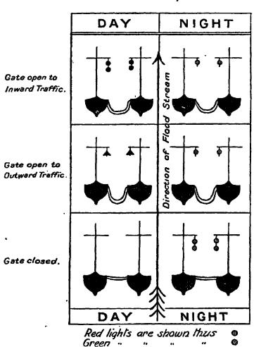
play signals, as shown on the accompanying diagram, to indicate whether the gate is open to inward or outward bound traffic, or whether the gate is closed.
